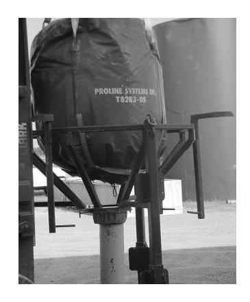
Thru the valve opening undo the nylon rope and the strap and unfold the bag's discharge throat.
