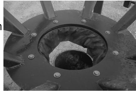
■ The crane lowers the bag into the rack, but remains 4 – 5 inches above bottom.
